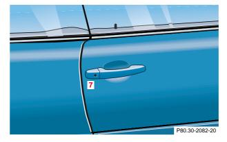
7 Infrared receiver in passenger door handle
